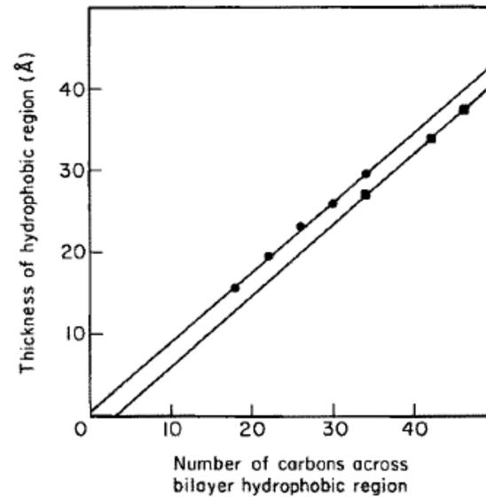
FIG. 3. Plot of the measured thickness of the bilayer hydrocarbon region *versus* the number of carbons across the hydrophobic region. The number of carbons is taken starting at C-2 of each acyl chain. Estimated errors in the thickness measurement correspond to the size of the plotted points. The lines are least-squares fits to the data. Circles, saturated acyl chains; squares, monounsaturated acyl chains.
