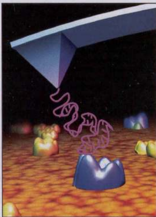
Figure 1. A schematic, not to scale, shows an atomic force microscope probe with attached aptamer scanning a surface. Because of its structure and chemistry, the aptamer alters the probe's response near particular molecules, enabling the location of that type to be mapped. Image courtesy of Stuart Lindsay, Arizona State University.
